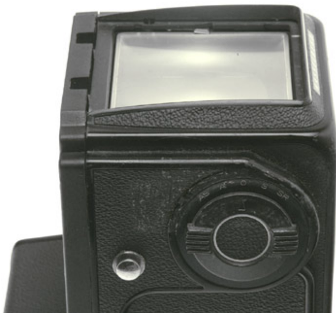
Camera top with cover removed, exposing the focusing screen
